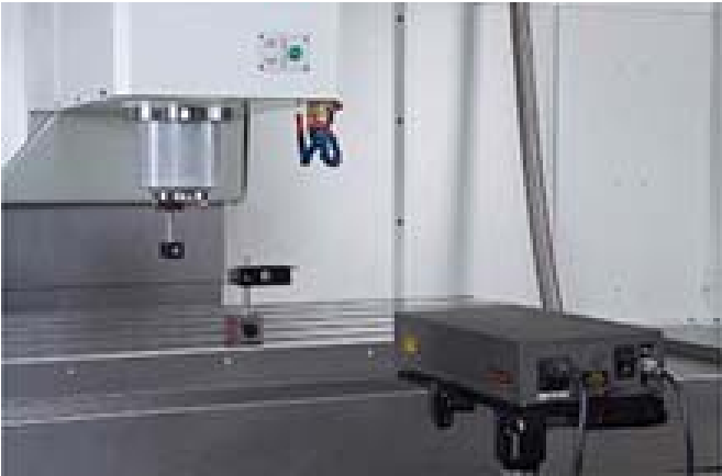
■ Laser Inspection for Linear Positioning Accuracy
